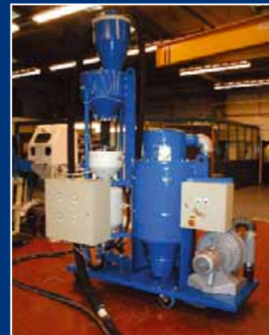
A very powerful continuous blasting P-08-2 fitted with vacuum pump recovery to reduce the air consumption
