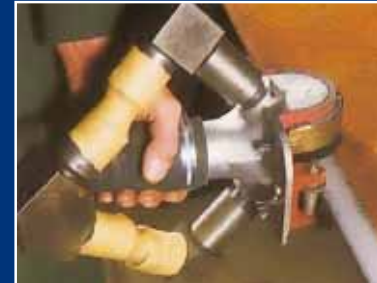
Plate edge gun. Cleans top, bottom and edge in one pass
